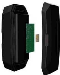
Embedded chip integration (Non-removable)
