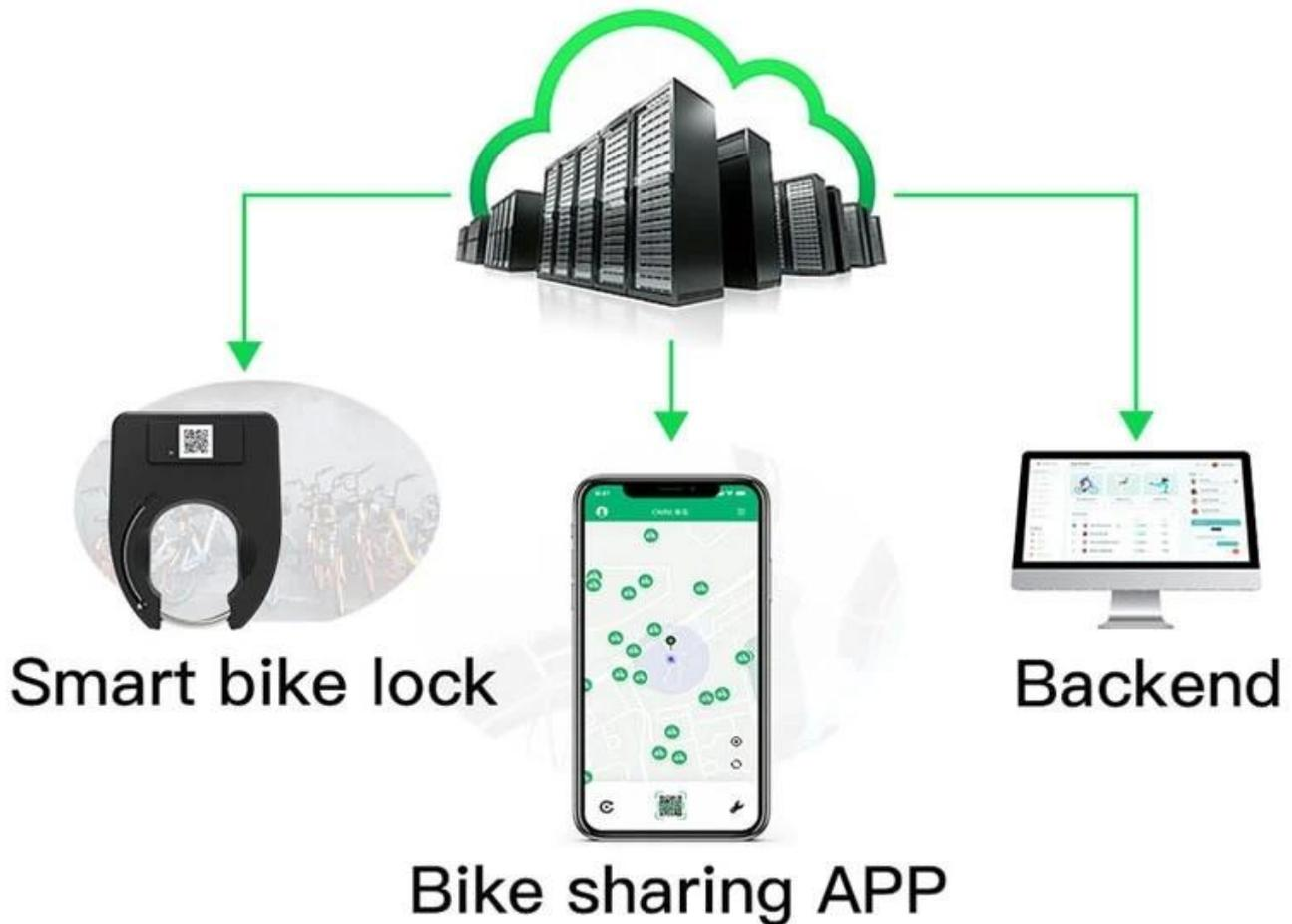
System architecture for a bike-sharing project. The system consists of a Cloud Server, Smart bike lock, Bike sharing APP, and Backend. The Cloud Server is connected to the Smart bike lock, Bike sharing APP, and Backend. The Smart bike lock is connected to the Bike sharing APP. The Bike sharing APP is connected to the Backend.
