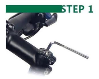
Release the original bead tube cap screw by allen key.
