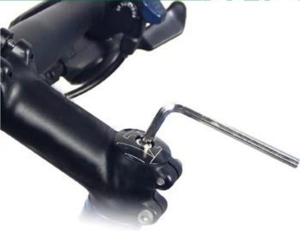
Release the original bead tube cap screw by allen key.
